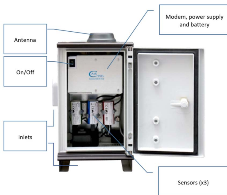
Figure 5.2 – Typical combined Dust, Noise and Vibration Monitor.
